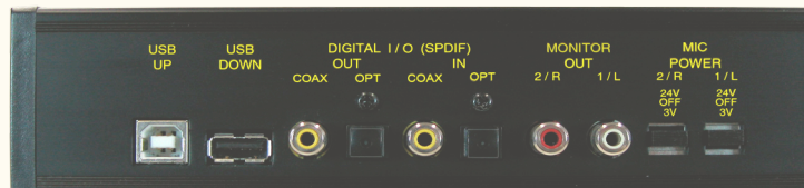
USB Connector Digital Input / Output COAX Optical x 2 Monitor Output 2/R 1/L Mic Power Switch
